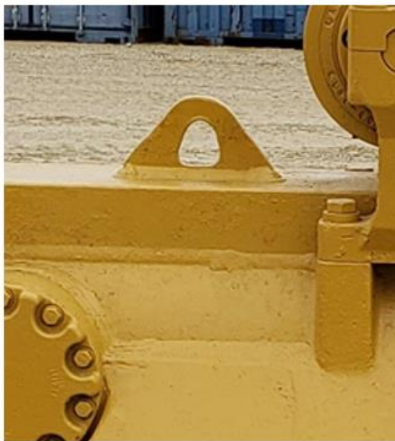
Example of a good lifting lug.
