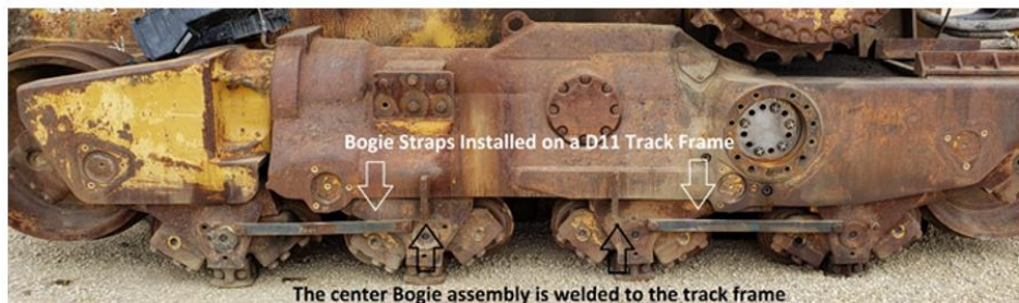
Bogie straps installed on a D11 track frame.
